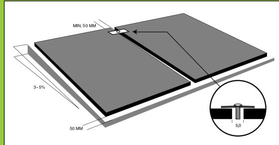
Installation using flat bar fittings. The method is mostly used in building conversions or in older buildings where the plastic mounting profiles are unsuitable.
